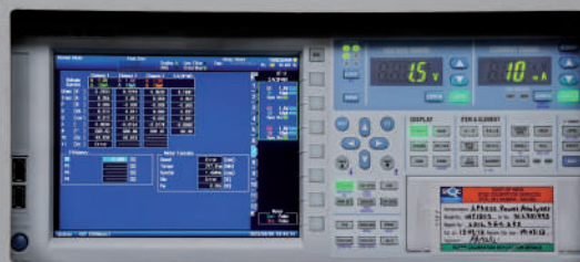
Efficiency determination as per IEC 60034-2-1 : 2024
