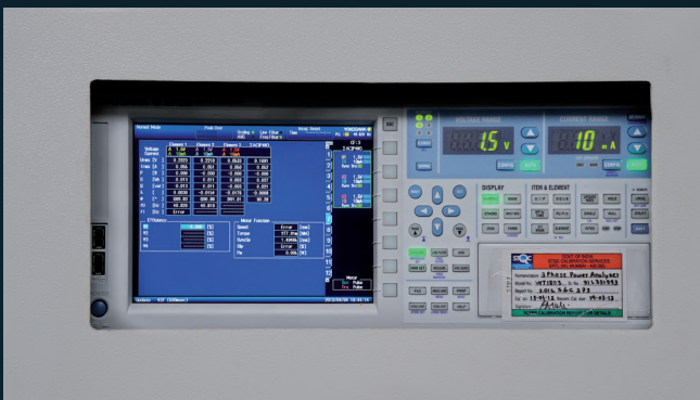
Efficiency determination as per IEC 60034-2-1: 2024
